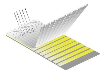
Fiber Type: E-Glass Architecture: 0°/90° Biaxial Dry Thickness: 0.055 in. / 1.40 mm Total Weight: 27.24 oz/sq.yd / 924 g/sq.m
